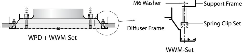
The WWM fixing set consists of 2 support frames, 4 spring clip sets and 4 M6 nuts and washers.
