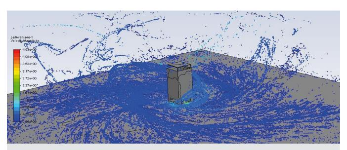
With the help of advanced numerical simulation (CFD), which was carried out in the OC IMP Klima R&D center, the exact air distribution pattern during the operation of the unit and filtration capacity could be determined. The results prove that one OC Air Purifier 1000 can efficiently filter air particles in rooms with up to 100 m<sup>2</sup> surface area while maintaining low noise levels and favorable air velocities.
